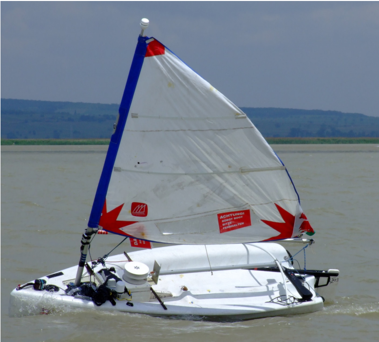
Figure 4.6: A photograph showing Pinta with its cut down sail and Bermudan rig.
