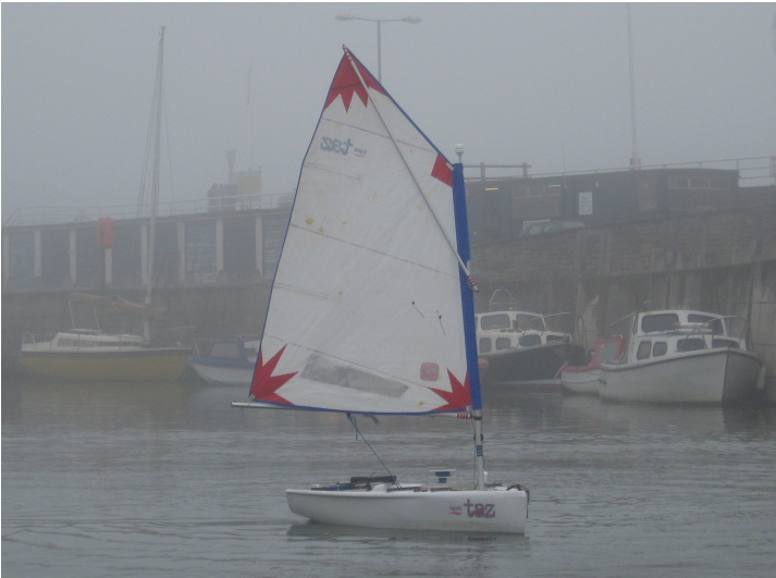
Figure 4.5: A photograph showing Pinta with its original sprit rig.
