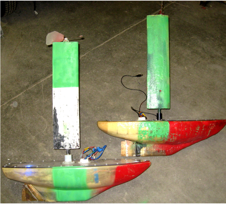
Figure 4.9: MOOP1 (left) and MOOP0 (right) out of the water showing the keel and rudder designs.
