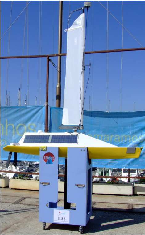
Figure 3.2: IBoat in 2009, the boat has been upgraded with solar panels, an ultrasonic wind sensor and a smaller sail.
