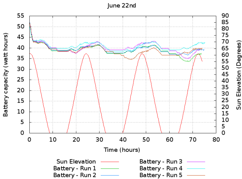
Figure 6.28: A graph showing sun elevation and battery levels during the course of the solar power simulation, running in June with an additional solar hormone.
