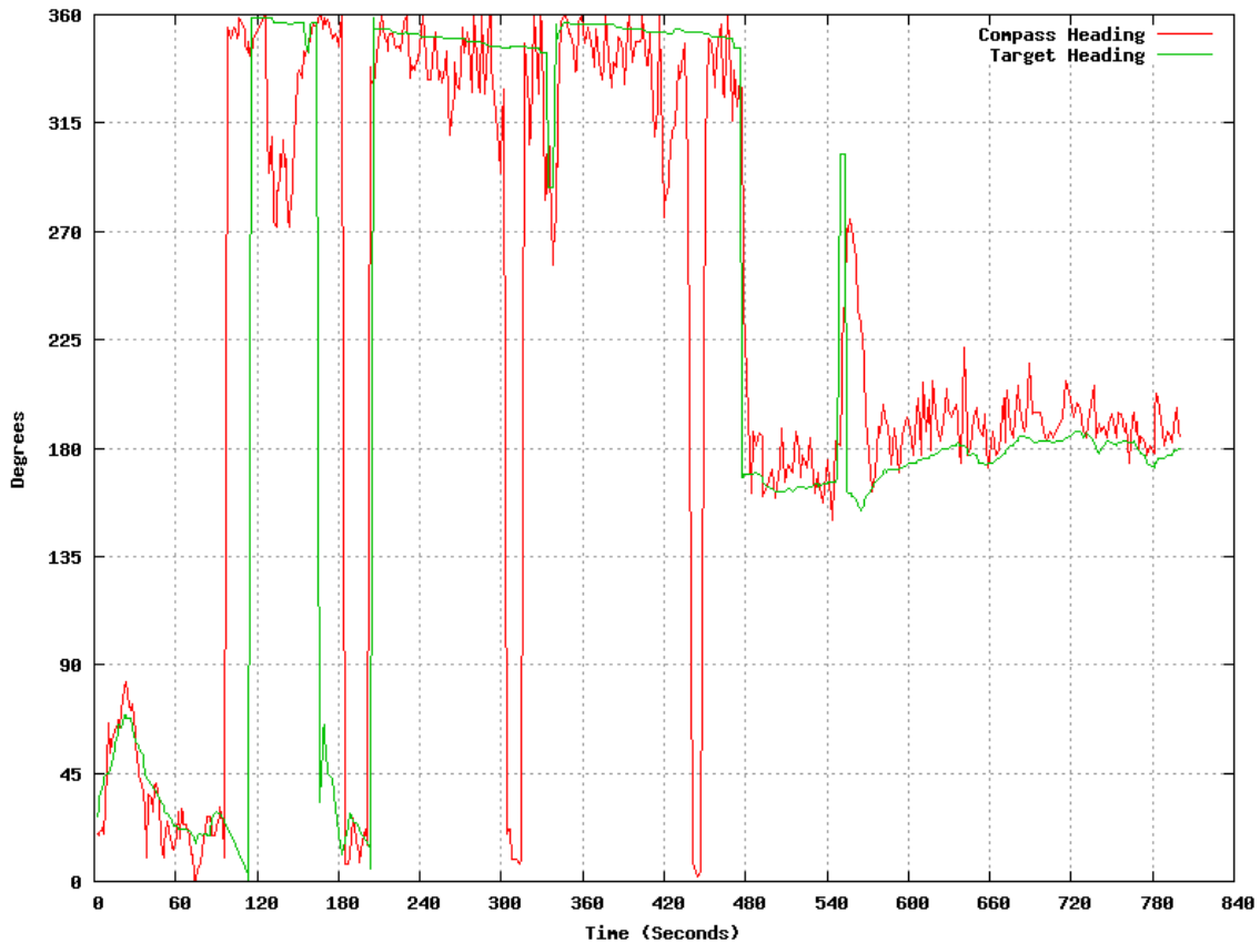
Figure 4.19: A graph showing the headings of a MOOP during the example course (the corresponding GPS trace can be seen in figure 4.18).
