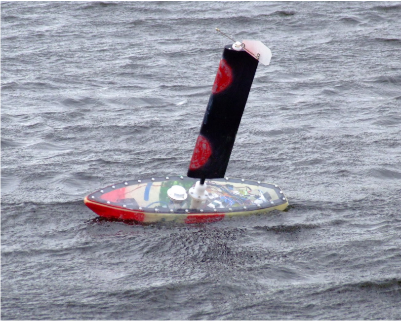
Figure 4.7: MOOP1 being sailed on a lake near Aberystwyth during initial testing and development work.
