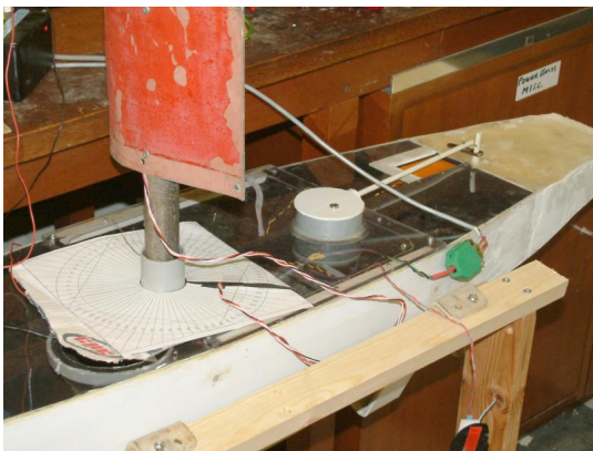
Figure 5.3: The setup for measuring the angle of the sail. A piece of copper wire is attached to the mast below the sail and facing the same direction as the sail, although its a bit difficult to see in this image. The piece of paper on the deck has angles marked out every five degrees, with zero degrees facing towards the front of the boat.
