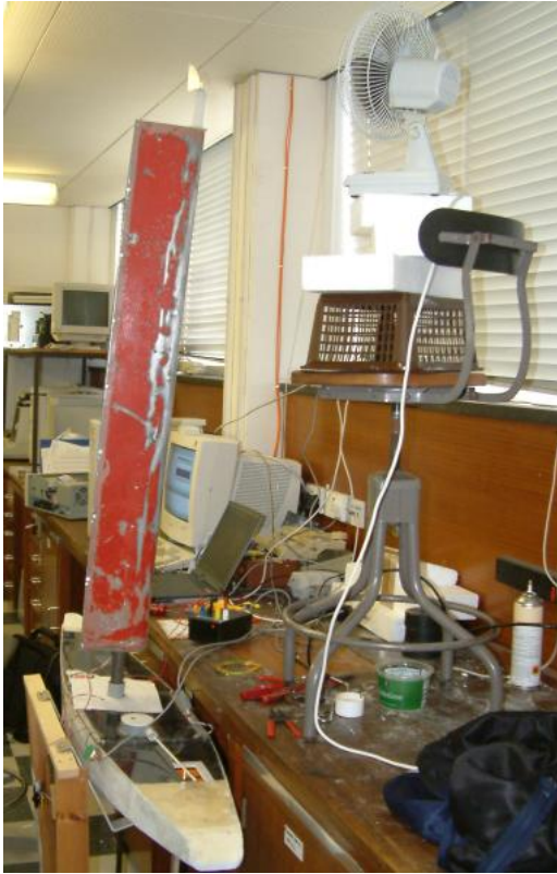
Figure 5.4: The setup for wind testing. The fan was later moved to be at 45 degrees to the boat.
