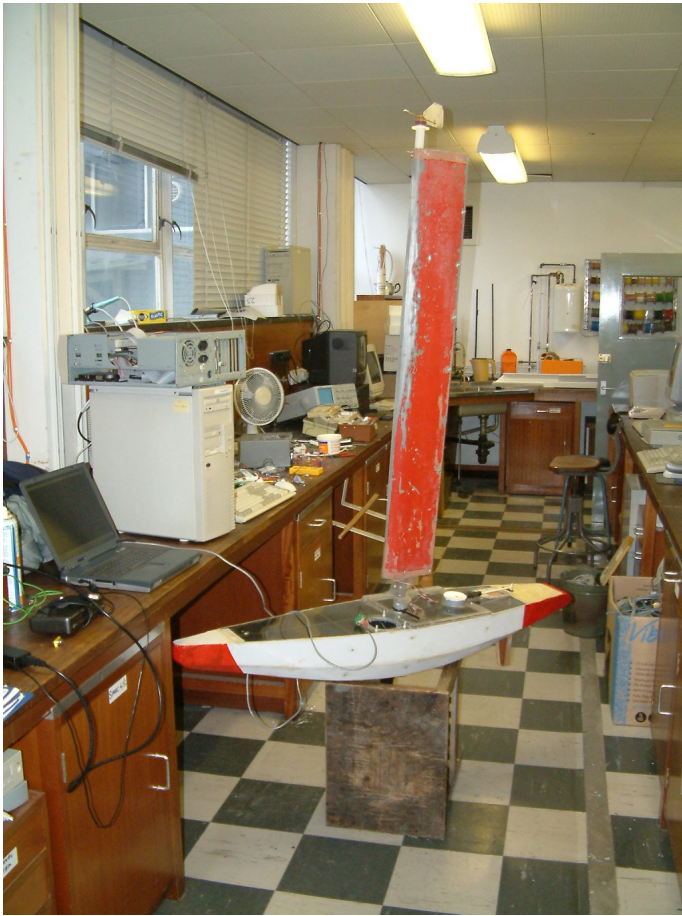
Figure 5.2: The compass calibration setup. By co-incidence the right side of the room shown is almost exactly magnetic north.
